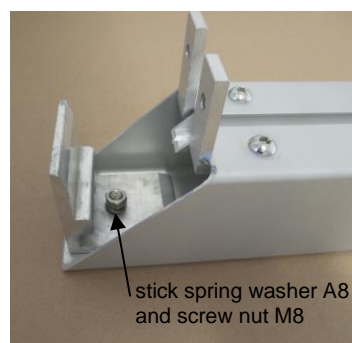
adjust angle parallel to bar outside edge
