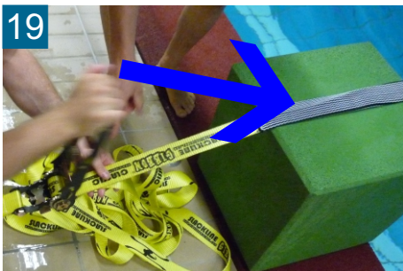
19 Look out for even alignment of abrasion protection
