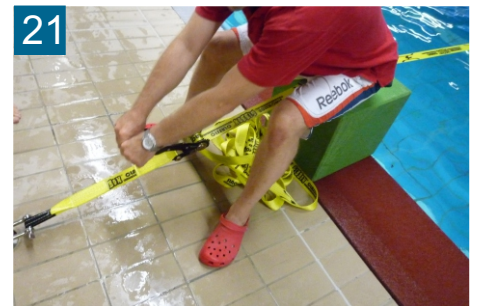
21 Adjust slackline manually Important: secure ratchet!
