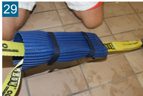
Fix ratchet cover with velcro fastener
