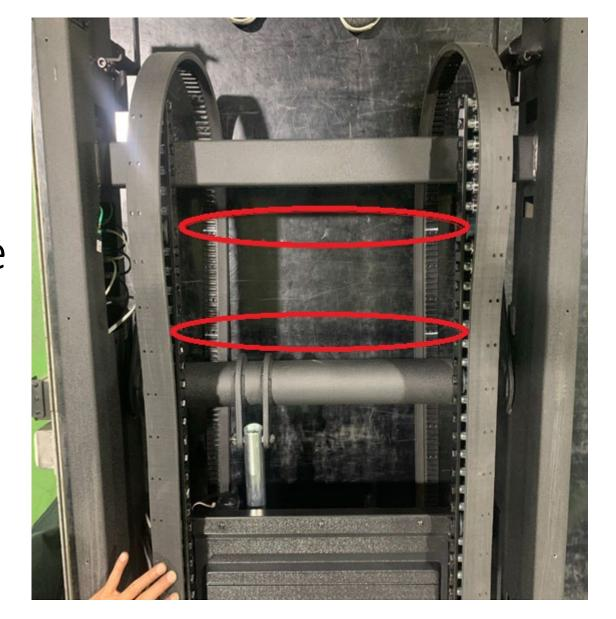
Step 5. Put the hole of timing belt in the middle groove that between rear roller gear and gear 將時規皮帶之打孔處置於後滾筒齒與齒的中間凹槽
