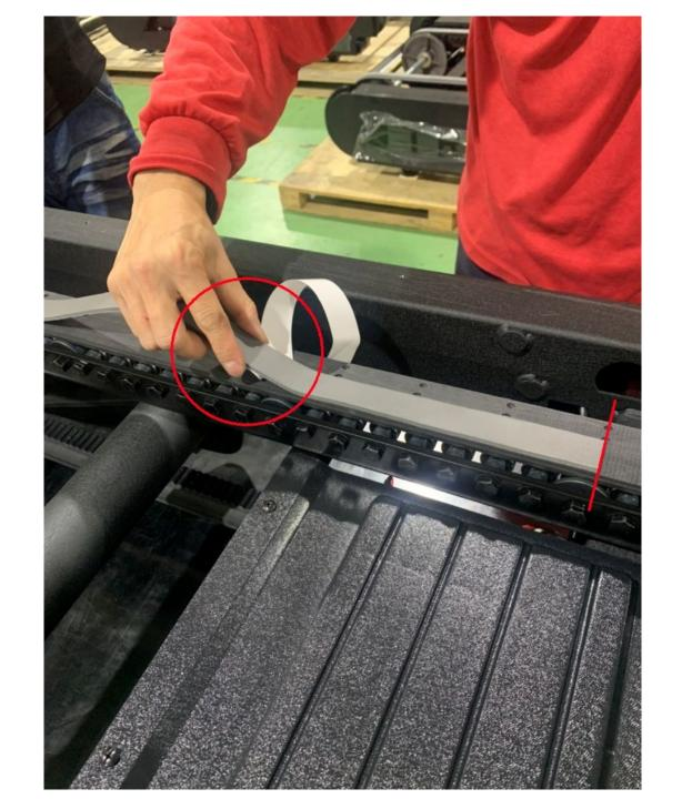
Step 9-1. Align to the hole then stick the rubber pad continuously (4 rubber pads on each timing belt) 以切齊孔位方式連續張貼泡棉(一邊時規需要四條泡棉)
