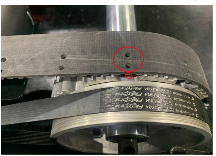
Step 6. Put in front roller and fasten the screw until front roller position is parallel with screw(look down from above) 放入前滾筒並將螺絲鎖緊,前滾筒位置約與螺絲平行處(正上方視角)
