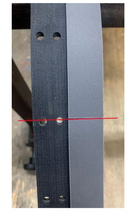
Step 9-2. We highly recommend rubber pad seam can exactly on half of the hole, this will be good look and not easily drop off.
