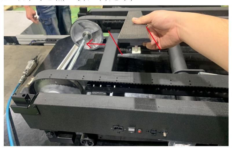
Step12(video). Put on no.95 pad plate and lock 96. nylon nut 放上鐵片,並繫上螺帽
