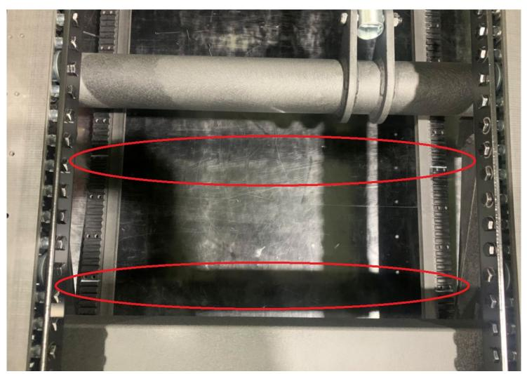
Step 8. Stick 93. BAM9000-250-30 rubber pad from the hole on timing belt. Please use same method to stick it, put them gently do not try to extend it. 貼上泡棉,請由時規上的孔處開始張貼,兩邊時規皆需保持相同的張貼狀況。張貼泡棉時,雙手以自然方式放置泡棉(參考手勢),勿拉伸泡棉
