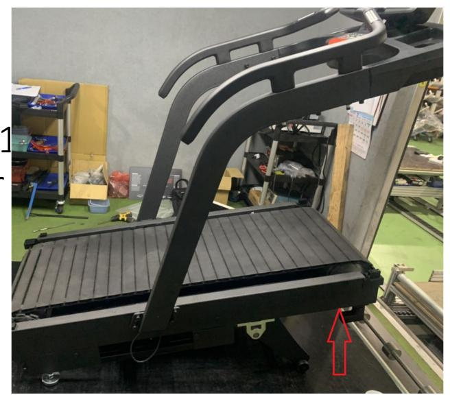
Step 3. Loose Incline strengthen round tube screw (no.248) near the wheel on left and right side 鬆開揚升補強桿螺絲(左右邊皆須鬆開)
