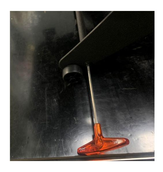
Step 4. Remove Incline strengthen round tube as following picture 移除揚升補強桿(建議兩側要撐開比較好拿)
