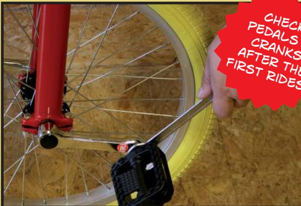
TIGHTEN RIGHT PEDAL CLOCKWISE AND LEFT ONE COUNTER CLOCKWISE. CHECK IF PEDALS ARE WELL TIGHTENED AFTER FIRST RIDE!
