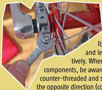
The pedals and crank-arms are handed; they are labelled "R" and "L" for the right-hand side and left-hand side, respectively. When fitting the left-hand components, be aware that they are counter-threaded and so must be turned in the opposite direction (counter-clockwise to tighten) to the right-hand components (clockwise).
